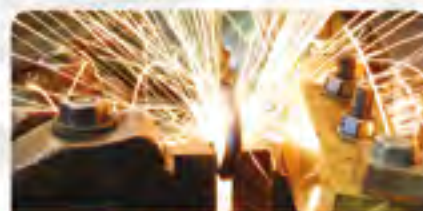
Flash Butt Welding
